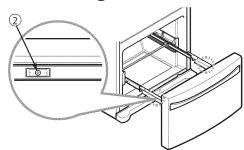
Grasp the drawer on each side and pull it up to separate it from the rails.
